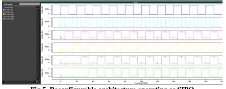
Fig.5. Reconfigurable architecture operating as SIPO
